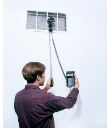
Rotating vane measuring an outlet
