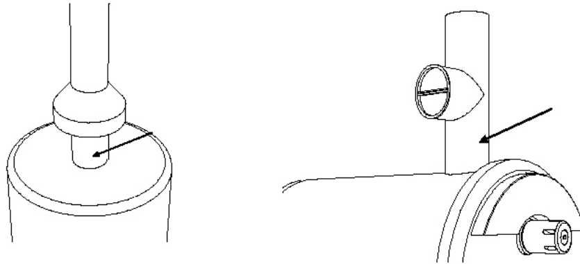
Flue Gas Sampling Locations
